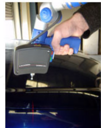
Fig. 2: ModelMaker Z70 mounted on a FaroArm
